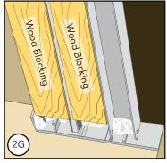
H. Set the wood blocking in sealant in the existing door frame. Make sure the blocking is flush with the furthest protruding part of the existing jamb. Place a 3/16" bead of sealant in the door panel cavities, then insert the wood blocking into the head cavities followed by the jamb cavities. Next insert the wood blocking into the jamb panel cavities of the existing door frame. Secure the blocking by pre-drilling and inserting #8 x 2-1/2" screws.
